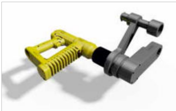
The 3D printed model can be assembled with the drive unit, which will be used later. So access of the entire system to the working area can be ensured.
