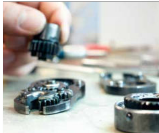
Below: Replacement of wearing parts in an open geared offset head.
